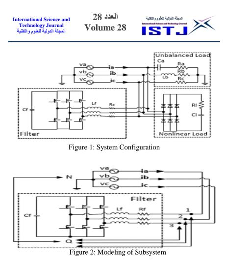
To investigate the rate of change of currents and voltages between the supply and the filter, Kirchhoff laws for current and voltage are applied. For simplicity, we consider the inverter switches are ideal; therefore, we ignore the leakage currents and the drop voltages on each IGBT.
