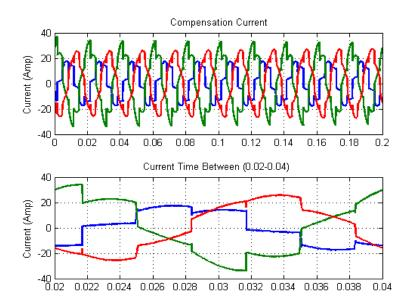
Figure 6: Compensation Current by the Filter
